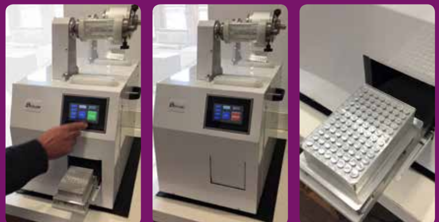
Figure 14: Random Access Sealing Procedure using the a45 RA Automatic Random Access Heat Sealer (4ti-0675, prototype shown)
